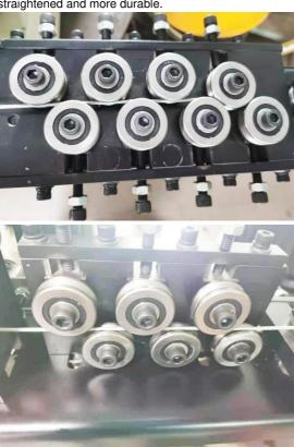
2. 4 groups, 8 wire feeding forming wheels, with large force, stability and wear resistance. There are only 3 groups and 6 similar machines from other manufacturers. Moreover, the processing is accurate, and the surface of the trunking is specially smooth.
